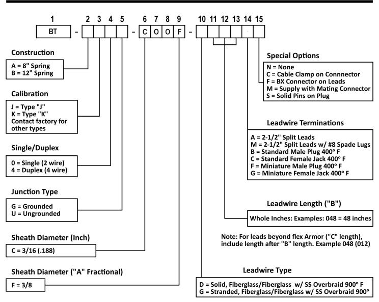
Note: Duplex and 1/8" OD sensors are usually constructed with 20 gauge wire. All others are generally constructed with 20 guage wire
